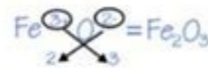
Figure 19.18: The criss-cross method is a simple way to determine the chemical formula of a compound.
